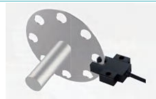
High-speed response of 3KHz for origin positioning and limit position Detect the holes in the rotary plate, read the number of revolutions and the speed.
