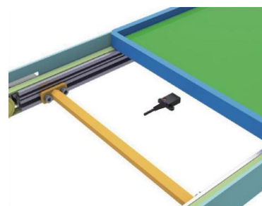
Confirmation of cardboard positioning and passing detection
